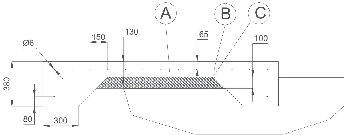
A: Concrete slab    B:Steel rod    C:Compacted sand
